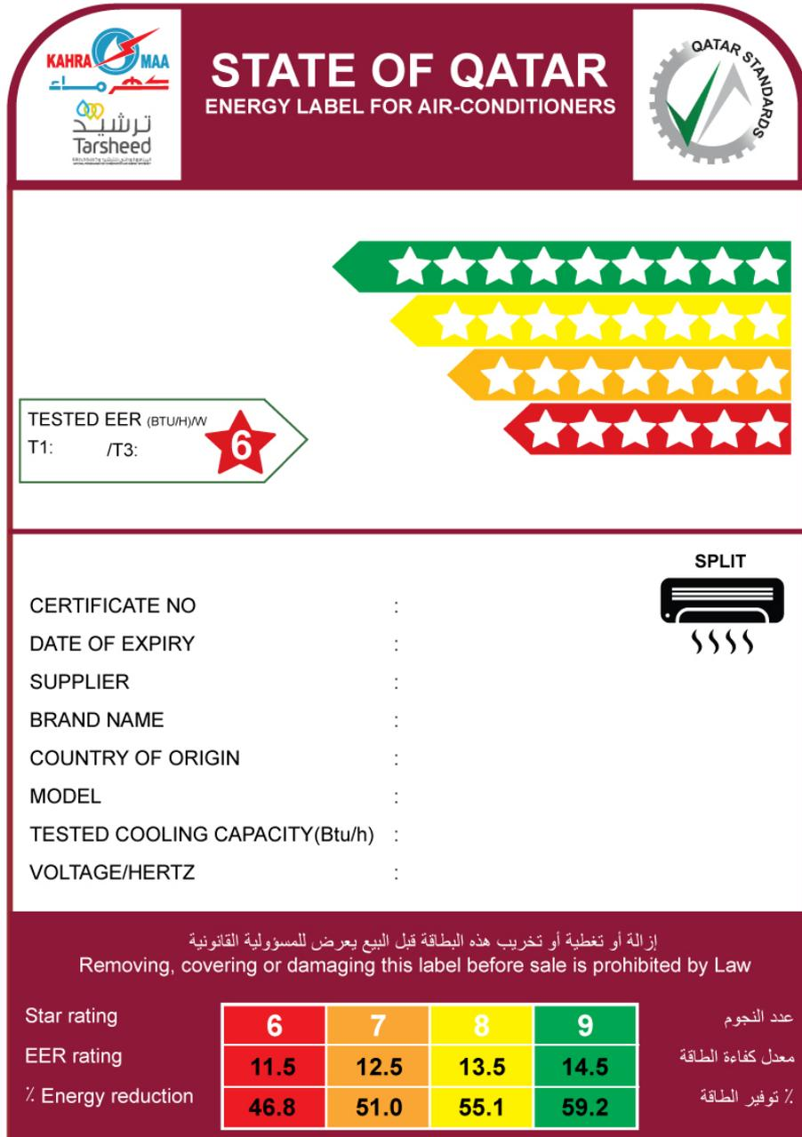
FIGURE 4: Example of Label for split type & Cooling Unit – 6 stars
