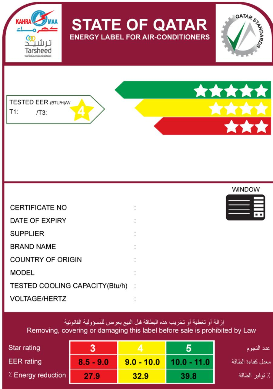
FIGURE 2: Example of Label For Window type & Cooling Unit – 4 stars
