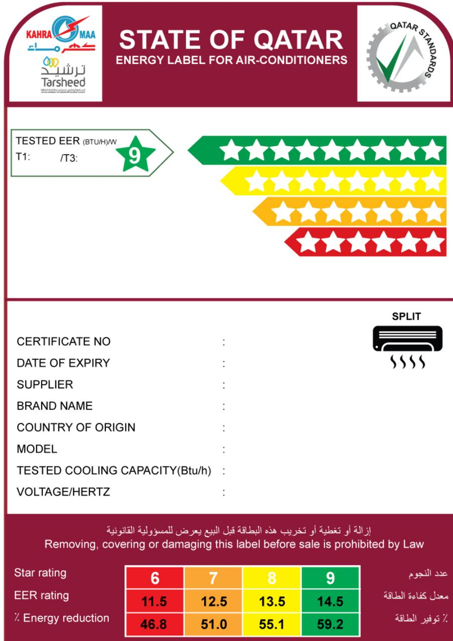
FIGURE 7: Example of Label for split type & Cooling Unit – 9 stars
